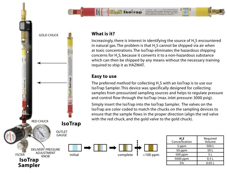
Flow until the indicator on the IsoTrap noticeably changes color. Remove and return to Isotech for analysis. No HAZMAT shipping is required.
